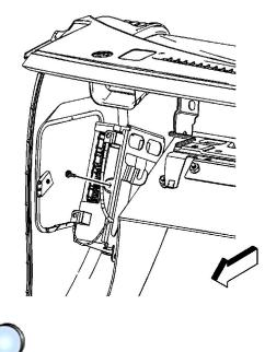
Remove the screw retaining the VCIM to the bracket.
