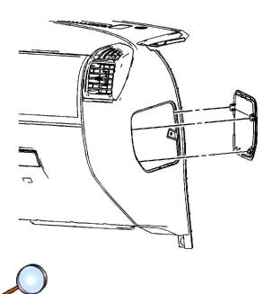
2. Remove the service panel located on the right side of the instrument panel (I/P).
