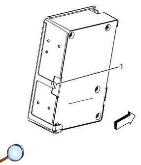
2. Install the VCIM to the bracket ensuring the retaining tab (1) is fully seated.
